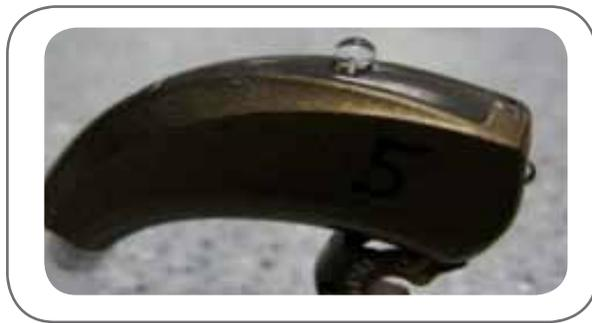
*Figure 6: HydraShield<sup>2</sup> still exhibits superhydrophobicity after two salt fog cycles.*
