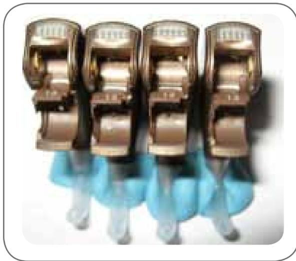
*Figure 7: No corrosion was observed in the battery compartment or DAI contact area after two salt fog cycles.*
