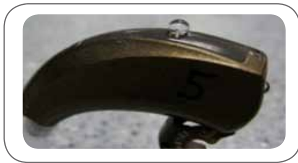
Figure 6: HydraShield 2 still exhibits superhydrophobicity after two salt fog cycles.
