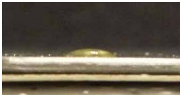
Figure 3: Photograph of a drop of olive oil on an untreated surface.
